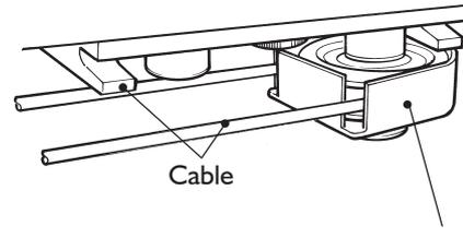
Clip stop end bolt removed and replaced with extended bolt, spacer and pulley assembly
