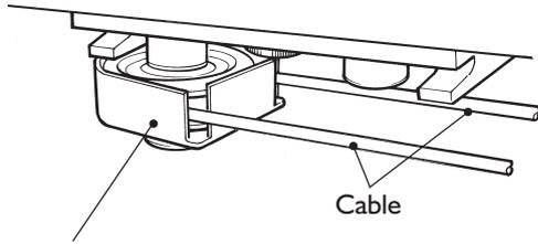
Clip stop end bolt removed and replaced with extended bolt, spacer and pulley assembly
