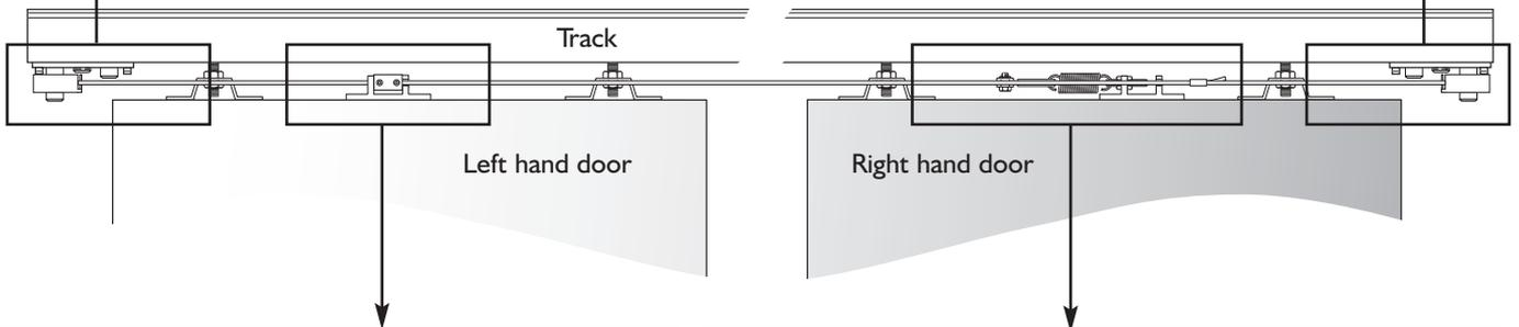
**Diagram 3. Cable anchored to left hand door**
